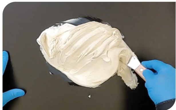
Combining parts A and B with a spatula using the folding method. Megapoxy PM should be streak-free, when fully combined.
