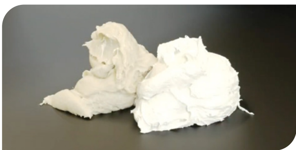
Measure out equal parts A and B by volume.
